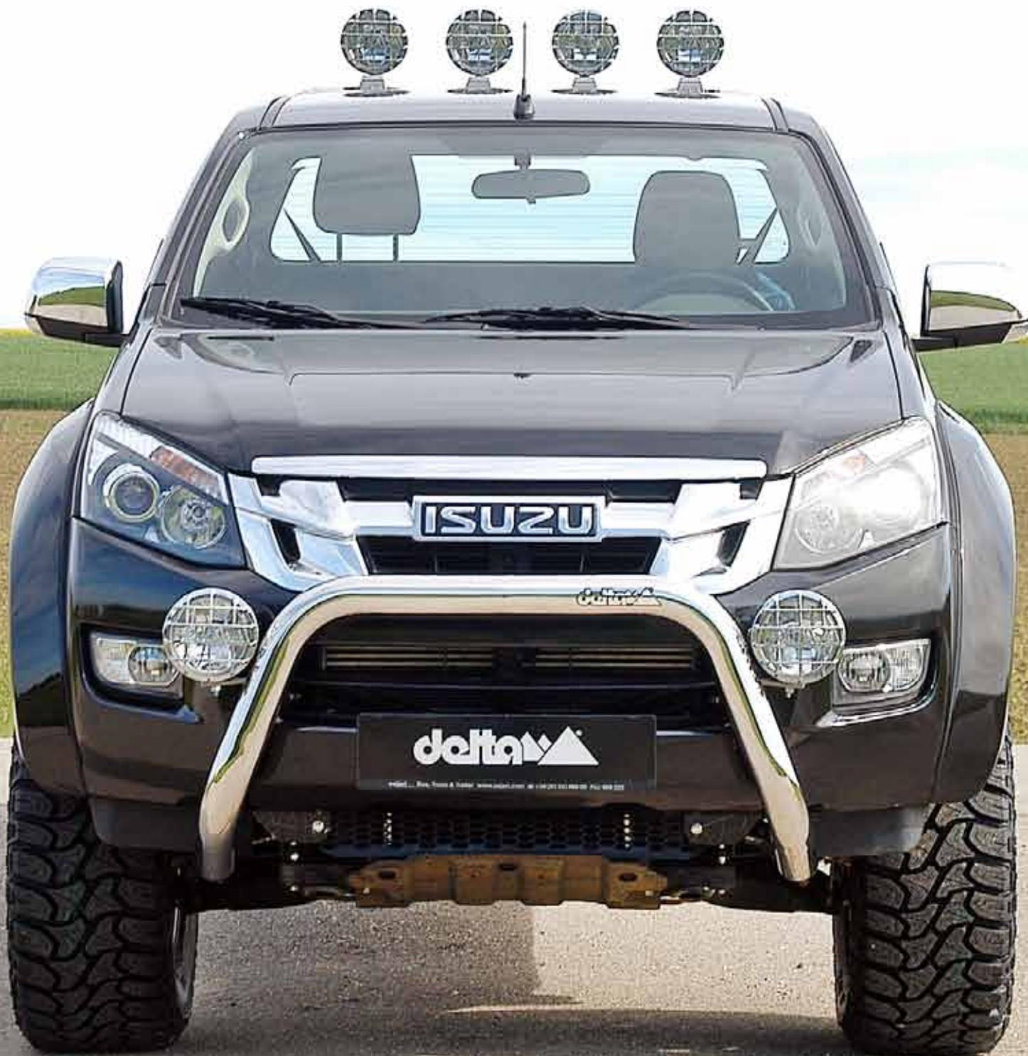
Frontbügel Edelstahl poliert 76 mm / Front bar stainless steel handpolished approved after EC pedestrian security law 76 mm
