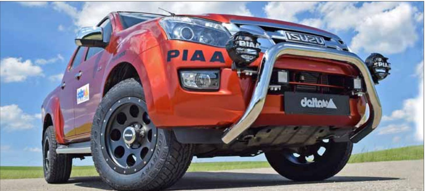
Frontbügel Edelstahl poliert 76 mm/Front bar stainless steel handpolished approved after EC pedestrian security law 76 mm
